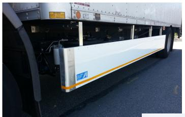
In response Allied Body Works, Inc. of Seattle has developed a truck side under ride guard that does not need to be custom built. Our guards combine safety and practicality. The design allows for installation on the majority of configurations within your fleet, and the adaptable design means that we can help create a solution, if they don't fit off the shelf.
